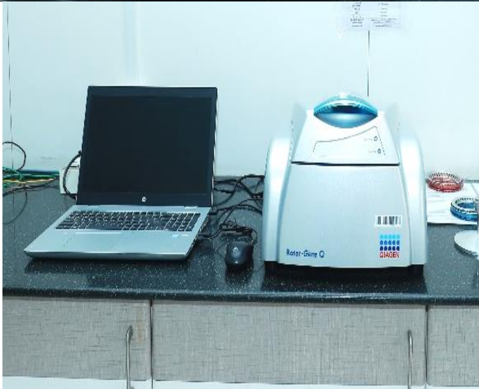
Conventional PCR machine and Real Time PCR machine with dedicated laptop for real time data analysis and report generation
